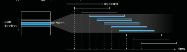
Exemplary illustration of the readout in line scanning mode with five exposure lines. This corresponds to a slit width of five times the pixel height.
